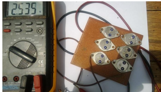
Figure 2. Voltage across four 2N3055 transistors
