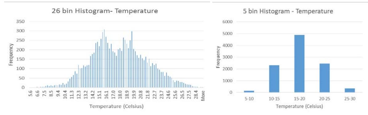
A histogram is a convenient way to summarize the data to identify statistical descriptors like minimum and maximum, while also allowing you to see the type of distribution of the data (uniform, binary, single peak, two peaks, normally distributed, etc). The histogram gives you an idea of the
